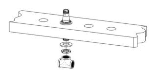
Apply plumbers' tape onto the bottom shank of the spout anchor. Secure the supplied tee connection to the bottom mount shank.
