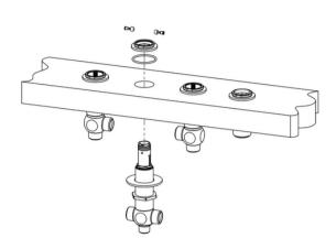
Secure in place from the bottom mounting nut.
