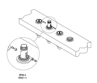
Fasten the roller and roller screw into place on both sides of the diverter valve.
