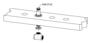
Ensure one of the divot holes is facing toward the direction of the tub.
