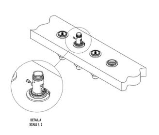
Tighten down the screw with a flat head screwdriver.
