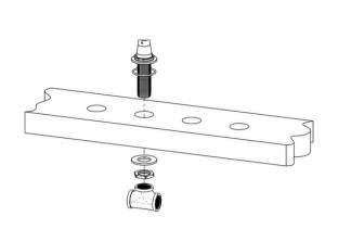
Place the spout anchor mount through the deck from the top of the deck.
