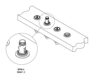
Attach hot/cold valve to diverter valve, utilizing  $\frac{3}{4}$ " connections.
