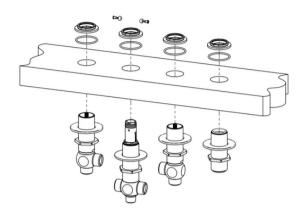
Disassemble top nut and o'ring seal from the top of the valves and cradle mount. 2
