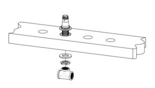
Secure the washer and mounting nut from underneath the deck.
