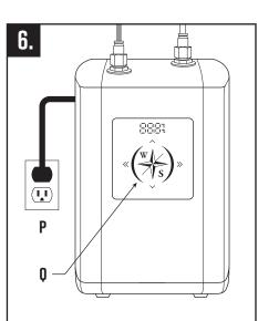
Check that installation area is dry and no water has spilled. Connect plug to the power socket (P). The Hot Tank's display panel (Q) will light up with the ON/OFF power button illuminated.
