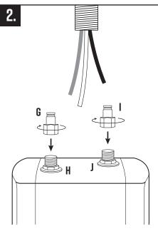
Attach quick connect fitting (G) to red Hot Tank inlet (H). Attach quick connect fitting (I) to gray Hot Tank outlet (J).
