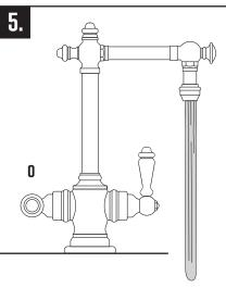
**DO NOT** plug-in unit until tank is full. Turn on faucet hot water until water flows freely. This means Hot Tank is full. Tank will take about **90 seconds** to fill. Turn off faucet and check all connections for leaks or hose kinks.
