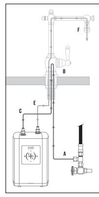
Water from the blue supply tube (A) flows through the faucet base to the ON/OFF valve (B). Water is then diverted into the red tube (C) and into the Hot Tank (D) and pressure is regulated through the built-in PRV valve. The inbound cold water displaces hot water in the tank causing it to flow freely through the clear "high temp" clear line (E). Hot water continues straight through the faucet and exits the spout (F).
