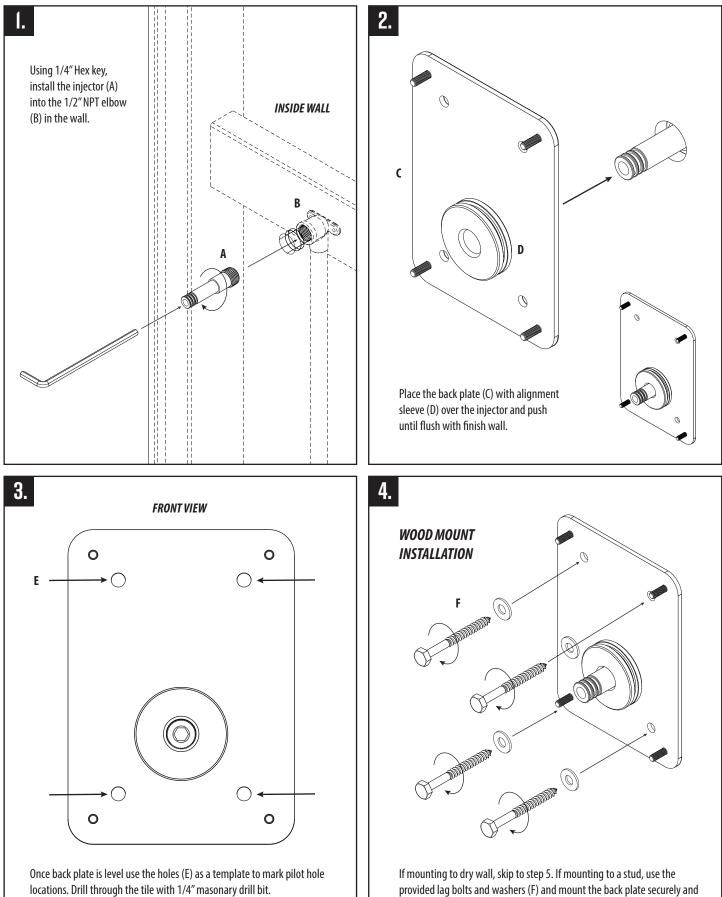
to the finished wall. Ensure plate is level.
