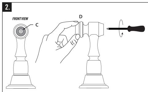
On the inside of the sprayer handle is a phillips retaining screw (C). Hold the sprayer button (D) in place with one hand and loosen the retaining screw with a phillips screwdriver.
