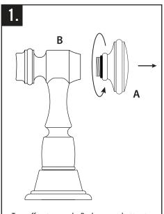
Turn off water supply. Push sprayer button to relieve water pressure. By hand, unscrew and remove spray head (A) from sprayer handle (B).
