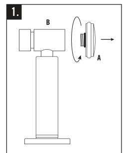
Turn off water supply. Push sprayer button to relieve water pressure. By hand, unscrew and remove spray head (A) from sprayer handle (B).
