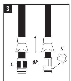
Slide latch connector up to expose compressor collar (C). Depending on hose configuration, there may be either a black collar or two brass metal circles.
