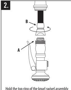
Hold the top ring of the knurl swivel assembly (A) with pliers. Use an adjustable wrench and losen latch connector (B). Remove nozzle.
