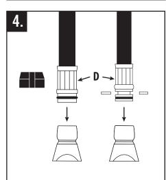
Carefully pry black collar off neck of hose connection (D). The half circles are loose and will just fall out. Slide latch connector off end of hose connection.
