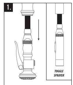
Turn off water supply. Open faucet to relieve pressure. Pull nozzle down from spout to expose swivel assembly.
