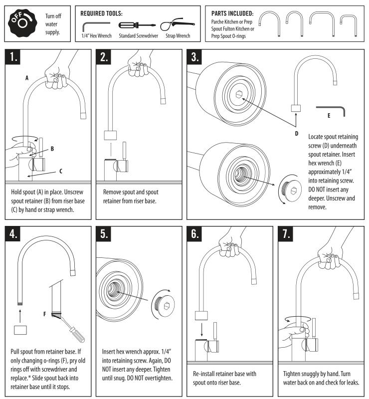
\*NOTE: IF REPLACING OLD SPOUT WITH NEW SPOUT, DO NOT REMOVE O-RINGS.
