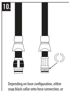
slide the half circles onto each side. Hold in place and slide latch connector down,
