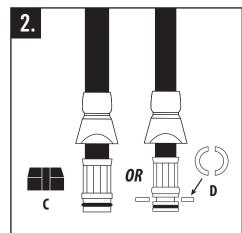
Slide latch connector up to expose compressor collar. Depending on hose configuration, there may be either a black collar (C) or two metal half circles (D). Carefully pry black collar off neck of hose connection. The half circles are loose and will just fall out.
