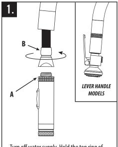
Turn off water supply. Hold the top ring of the knurl swivel assembly (A) with pliers. Use an adjustable wrench and loosen latch connector (B). Remove nozzle.
