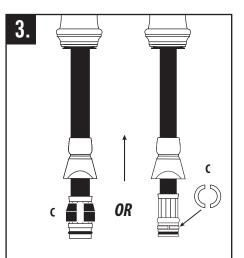
Slide latch connector up to expose compressor collar (C). Depending on hose configuration, there may be either a black collar or two brass metal circles. Remove compressor collar.
