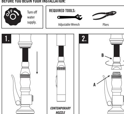
Turn off water supply. Open faucet to relieve pressure. Pull nozzle down from spout to expose swivel assembly.
