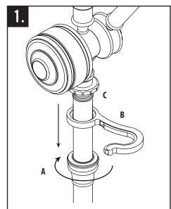
TURN OFF WATER SUPPLY! To avoid scratching finish, wrap the faucet riser with a sheet of paper. Unscrew retainer sleeve (A), by hand, until disengaged from thread. Carefully slide sleeve and spray hose hook (B) down to expose swivel threads (C).
