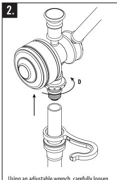
Using an adjustable wrench, carefully loosen the swivel unit (D). Unscrew by hand and remove Gantry sprayer head from faucet riser.
