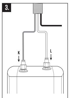
Before connecting tubes, checks ends for any sharp edges. Carefully push 1/4" red tube (K) into red inlet fitting until it hits the bottom and is secure. Repeat process with 5/16" clear tube (L) into gray outlet fitting.
